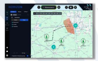
Dispatch applications can track multiple user locations and travel routes with job site time stamps to manage and dispatch vehicle fleets and remote workers. Dispatchers can draw geofences on the map to define boundaries for territories and service areas. Alarms can be generated when users enter or leave geofenced areas.
