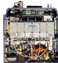
MR3332S-3 Internal Duplexer, 5 MHz separation
