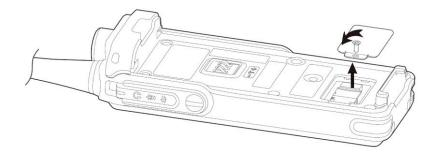
Install the TF card, put the card slot cover back in place, and then tighten the screw.
