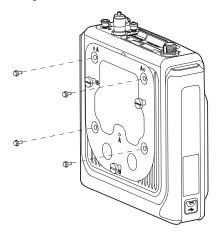
3. Install the repeater on the wall.
