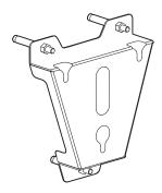
d. Dock the three holes on the bracket with the three pegs on the back of the repeater.
