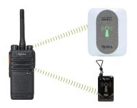
The PD412i can read and transmit RFID tag data. Used with the Hytera Patrol System, this radio provides real-time tracking and management of security personnel and resources.
