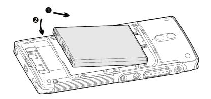
3. Press the cover into place and slide the battery latch to the lock position.
